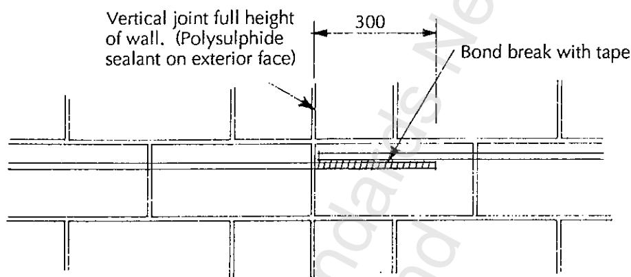
(a) Control joint separating two walls
