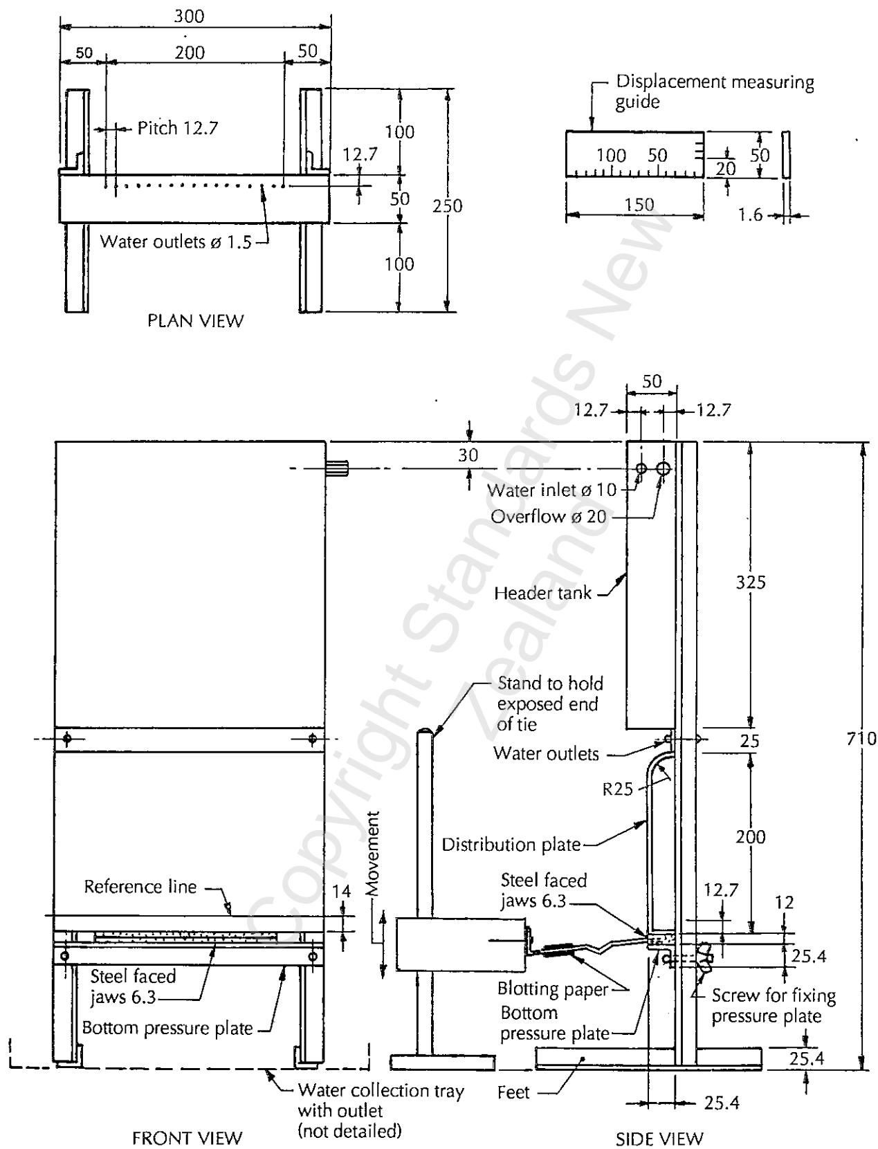
**TEST APPARATUS FOR RESISTANCE TO WATER TRANSFER TEST**
