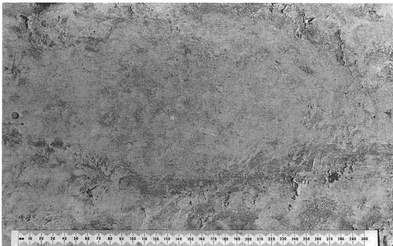
Fig. 7 PHOTOGRAPH OF TYPICAL SURFACE ILLUSTRATING CLASS F3 OFF-THE-FORM FINISH
